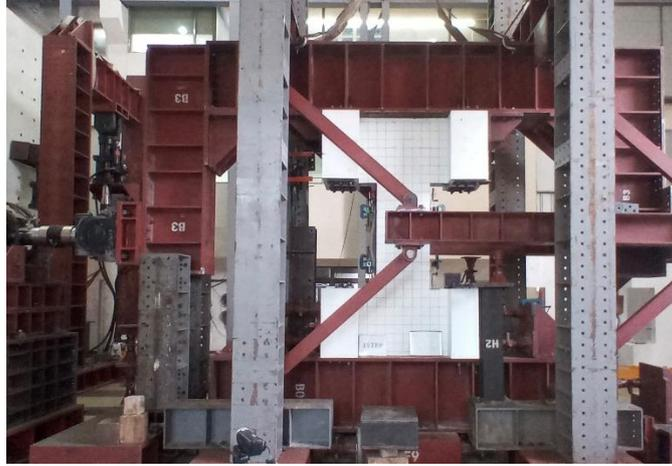
Fig. 2 Test set-up for coupling beam
