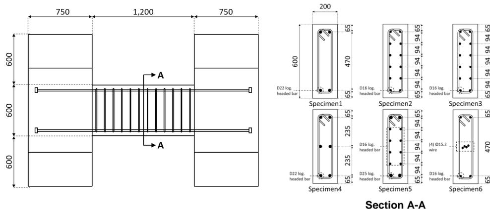
Fig. 1 Test beam geometries
